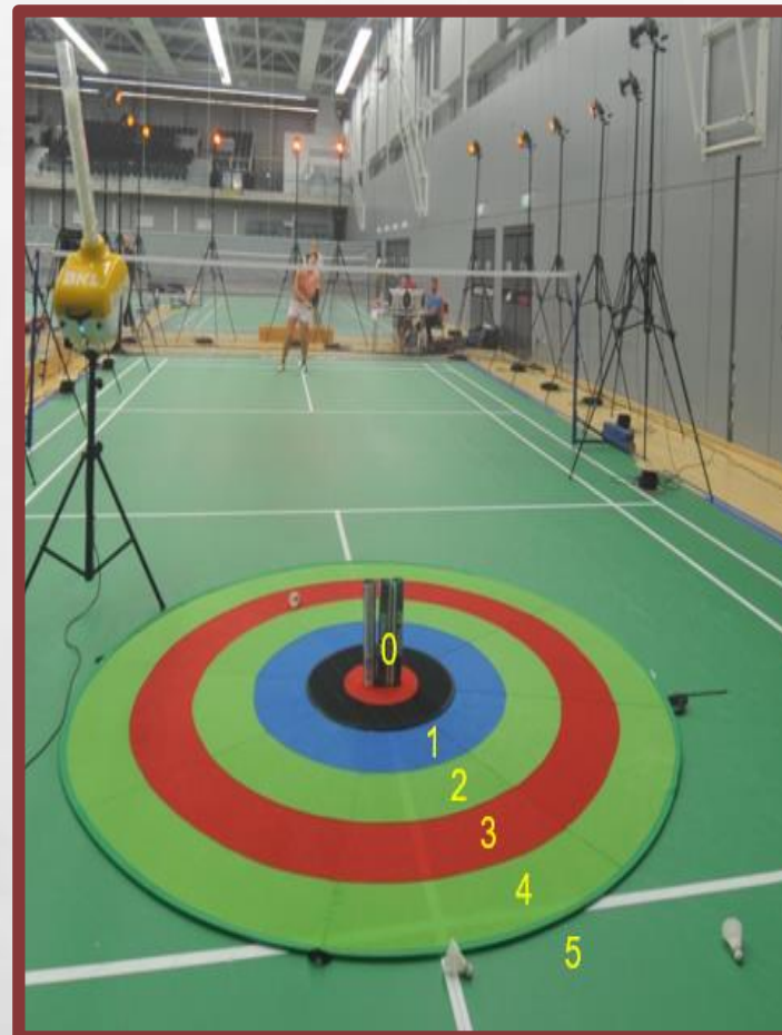
Figure 1. 3D motion capture setup; flat target and shuttlecock tubes
